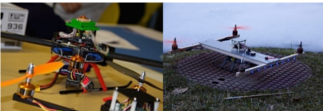
Picture 3: Two built models of the quadcopter. The first one made out of aluminum using a set, the second one built from scratch using wood. Both were built during the pilot workshop in Bad Hofgastein, Salzburg, Austria.
